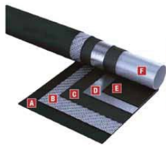
Key Features A Synthetic rubber cover B Braided reinforcement C Synthetic rubber layer D Aluminum foil layer E Synthetic rubber layer F Polyamide inner layer
